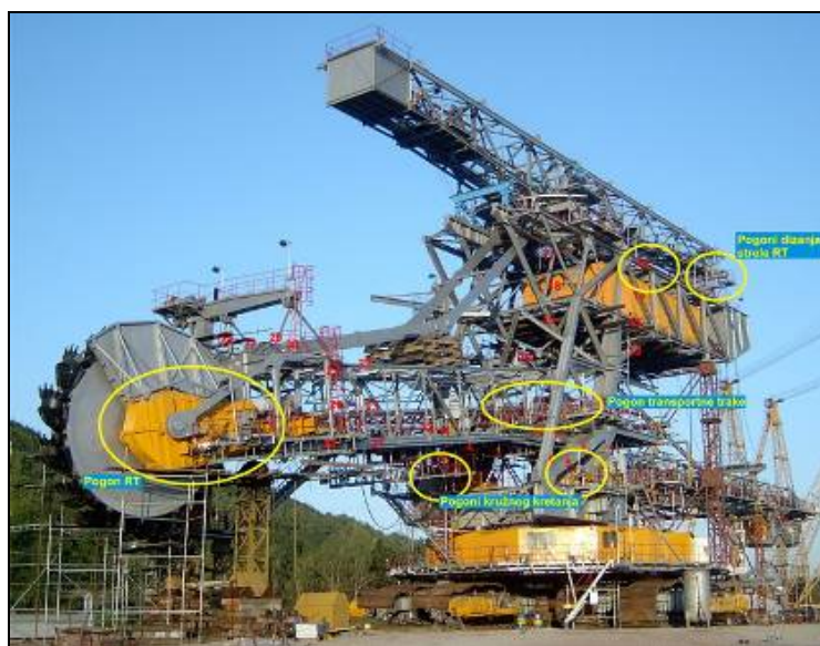
Figure 6. Measurement locations for strain (red circles) and vibration (yellow circles) measurement
